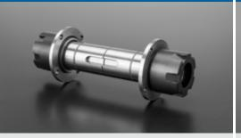
The frontal driven tool-holders are installed simply by screwing them into their lodgments. No belts or other special transmission systems are required. The maximum speed is 8,000 RPM.
