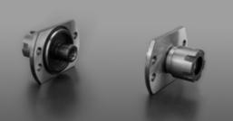
Static frontal tool-holders can be installed in any station of the rack, including stations designed for accommodating driven tools. This makes it possible to install a driven tool for machining the part carried by the main spindle and a static tool for machining the part carried by the pick-up spindle (or vice versa) in the same station. The tool-holders accommodate standard ER 20 collets.
