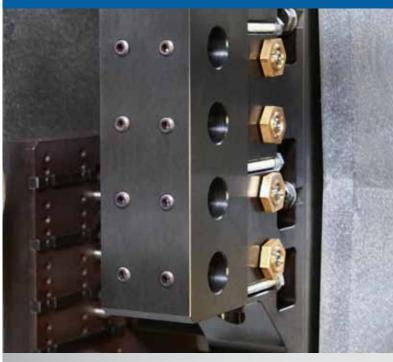
A tool rack with  $2\times 4$  stations makes it possible to perform distinct frontal operations simultaneously (i.e. centering, drilling or tapping) on parts carried by the main spindle or the pick-up spindle.
